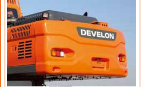
LOW CENTER OF GRAVITY DESIGNED COUNTER-WEIGHT
