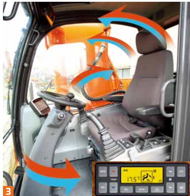
3. AIR CONDITIONING WITH CLIMATE CONTROL
